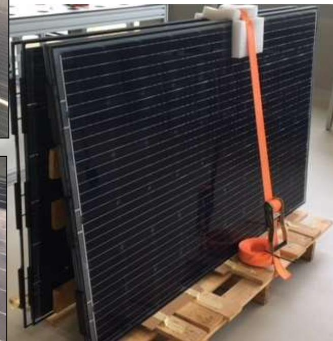
**2018:** 60-cell (5 pcs) and 9-cell (12 pcs) **BIPV modules** benchmarking of latest ribbon and industrial and imec multi-wire interconnection technologies
