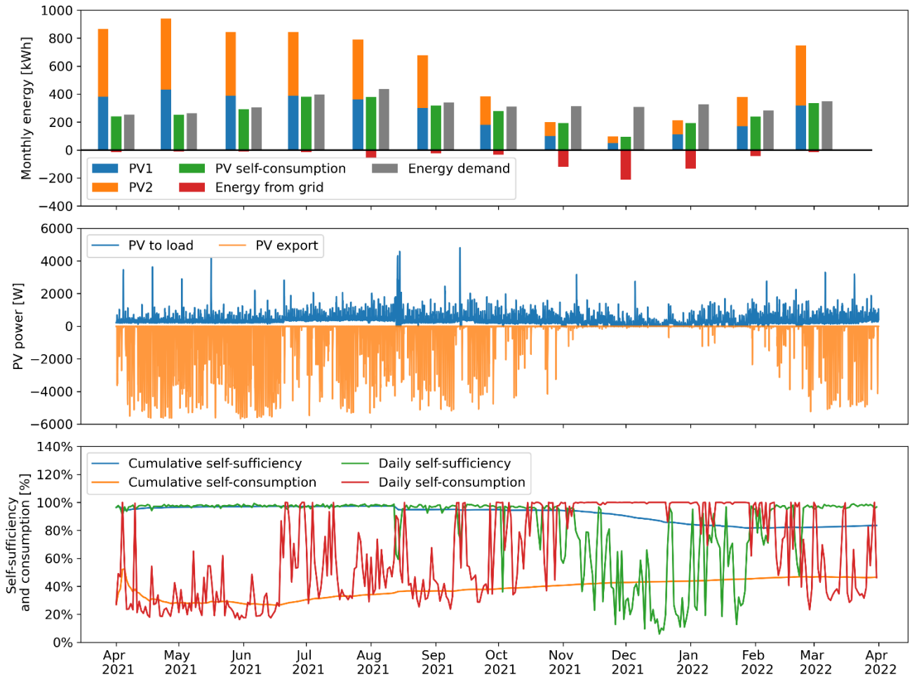
Figure 4: Total monthly energy generation and consumption (top pane), hourly PV power to load and export (middle) and daily self-sufficiency and self-consumption values for Groenhagemolen
