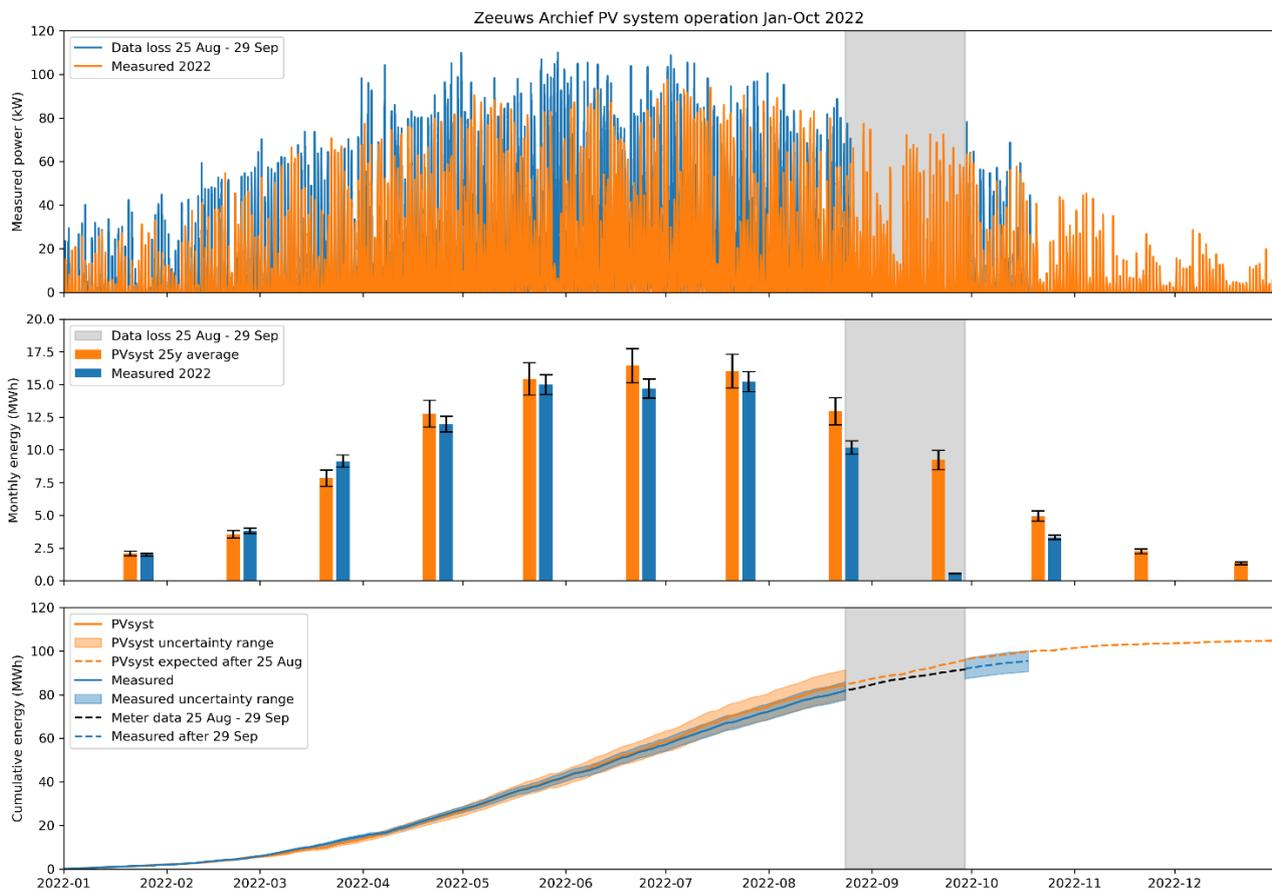
Figure 2: Zeeland Archives measured PV performance versus modelled by PVsyst. The data for 25 August to 29 September has been corrected using metering data (daily totals), as shown in Figure 3
